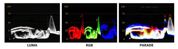
Figure 5.1-17 LUMA Waveform and RGB Waveform and PARADE Waveform
