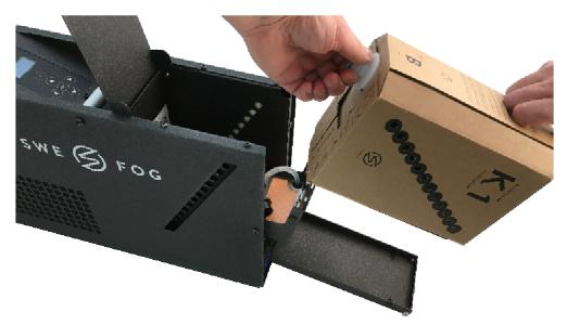
• The spout flange shall be positioned in the rail, <u>between</u> the black & stainless metal plates. Push in spout to center position.
