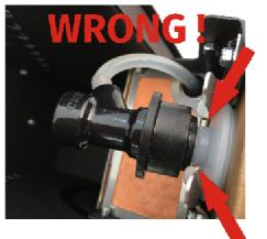
NOTE: Incorrect connection will cause fluid to leak out !
