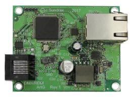
OEM board for integration into your fixtures and installations. ArtGate Compact OEM converts DMX512 to ArtNet/sACN in both directions. Various merging modes available: HTP, LTP, AUTO, PRIORITY, OVERLAY. Comes with optional RJ-45 to XLR output adapter. Compatible with any hardware and software supporting ArtNet and sACN protocols. Configuration is performed through web-based management page. Available as non-OEM package to be integrated into stage floors or wall sockets.
