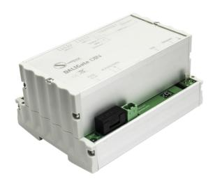
DALIGate DIN is DIN rail mounted converter that converts ArtNET/sACN/DMX signal into DALI protocol to include DALI lighting fixtures into controllable lighting network.
