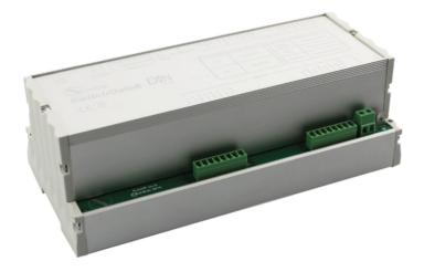
Din rail mounted DMX switch relay switch designed to switch 8 power circuits by DMX commands. Provides diagnostic feedback from 16 AC inputs via RDM.
