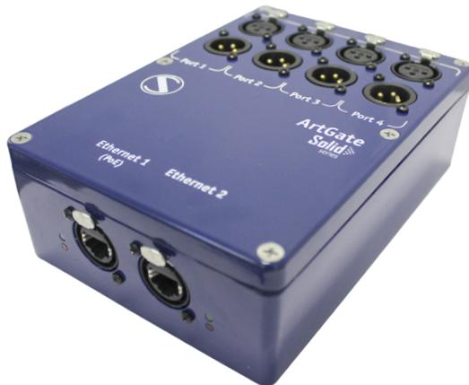
Multifunctional converters that translate Ethernet protocols (ArtNet, sACN) into DMX to control more lighting fixtures through single Ethernet LAN 10/100Base-T link. Incredible amount of universes thanks to second Ethernet port adding cascading availability through integrated switch. All DMX ports may be used as inputs or outputs.
