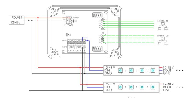
When using **12-48V** power source, set the jumper at **X3** connector. When using **5V** power source, jumper is **not** installed.
