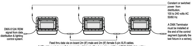
A 12' cable run between fixtures can be obtained without requiring additional DMX-512A data cables
