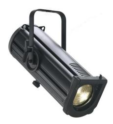
The PLFRESNEL1 is a general purpose luminaire for theatre, small studio, and display lighting applications. It produces an adjustable cone of light with a soft edge which is easily blended with adjacent beams to provide even illumination. Using LED source technology combined with a traditional Fresnel lens, the PLFRESNEL1 delivers Philips Selecon's industry benchmark quality without the compromising performance of spreader lenses.
