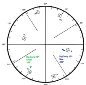
The position of the DigiComp HD Blue & Green signals on the vectorscope indicate the high level of chrominance and luminance that are crucial for a successful matte. The open squares shown on this diagram indicate the points at which chrominance and luminance are maximized.
