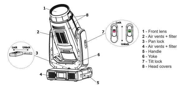
The head should be locked for transportation - the tilt lock (7) and the pan lock (3) have to be in the locked positions. To unlock the head, move these latches to unlock positions before operating the fixture.
