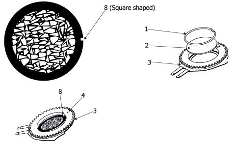
11 Insert the gobo holder back into gobo carousel in this way, that its position point (4) (or magnet (9) has to exactly aim at a small toothlike projection (5) on the edge of the rotating gobo wheel. Do not move with neighbouring gobo holders.
