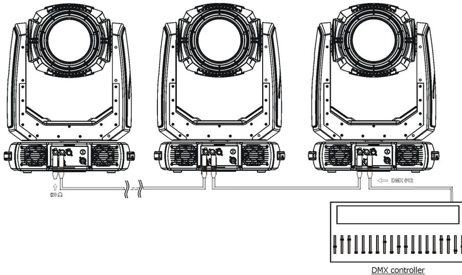
Connect the DMX-output of the first fixture in the DMX-chain with the DMX-input of the next fixture. Always connect one output with the input of the next fixture until all fixtures are connected. Up to 32 fixtures can be connected.
