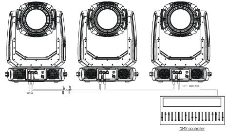
Connect the DMX-output of the first fixture in the DMX-chain with the DMX-input of the next fixture. Always connect one output with the input of the next fixture until all fixtures are connected. Up to 32 fixtures can be connected. **Caution:** At the last fixture, the DMX-cable has to be terminated with a terminator. Solder a 120  $\Omega$  resistor between Signal (-) and Signal (+) into a 3-pin (5-pin) XLR-plug and plug it in the DMX-output of the last fixture.
