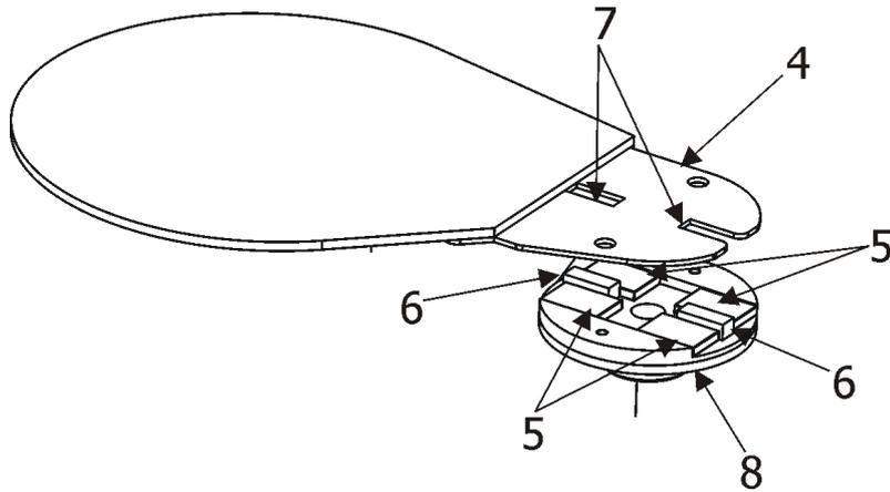
6. Insert a new frost module into the frost holder (8). Check, that both slots (6) snapped correctly into two protrusions (7) on the holder (4)
