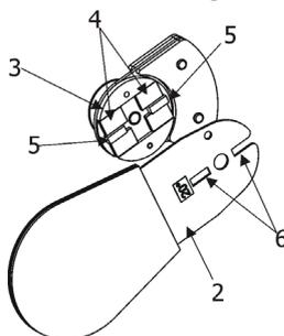
4. Place a new frost module into the frost holder (3). The glass heat filter has to face towards the light source (LED module)! Check, that both slots (6) snapped correctly into two protrusions (5) in the holder (3).
