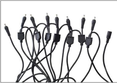
The DMX PSU enables up to 24 Apollo lights to be powered from the mains and dimmed under DMX control. Lights are connected to the PSU by 3 bud chains, each connecting 8 lights. Each bud chain can be dimmed independently. The bud chain plugs have a twist lock which prevents accidental disconnection.
