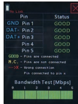
DMX Cable Test
