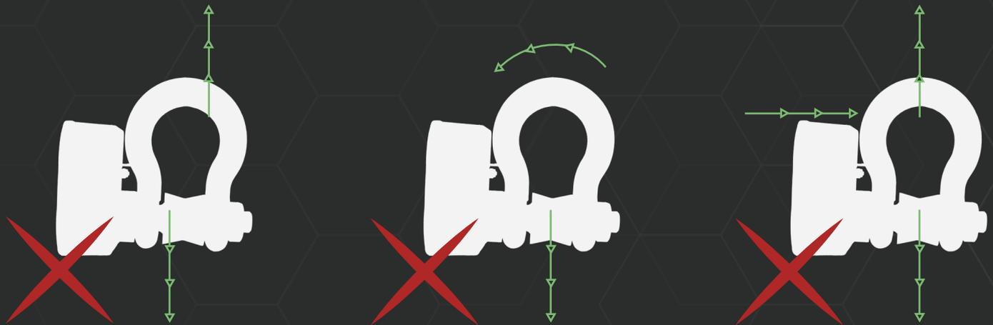
The end fitting of the steel wire or, for example, the hook of the chain hoist connected to the Load Cell shackle must allow the bobbin to centre the position of the end fitting or hook. Otherwise use an additional shackle to connect the steel wire of chain hoist hook to the Load Cell shackle
