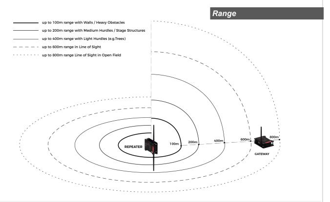
In case it is necessary to cover longer distances or there are large obstacles to overcome, it is possible to add Repeaters, which can be located as far as 600 meters from the cells and 700 meters from the Cateway. It is not possible to connect multiple Repeaters in series: each Repeater needs a direct connection to the Cateway
