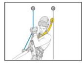
The ASAP'SORBER AXESS allows the rope to be kept at a distance to protect it during certain work phases.
