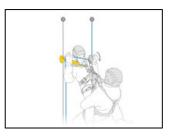
The ASAP'SORBER AXESS can be used for loads up to 250 kg in two-person rescue situations.
