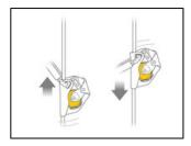
In normal use, the ASAP mobile fall arrester moves freely along the rope to accompany the user in all his movements.
