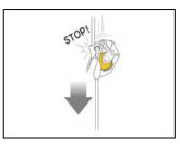
In case of a sudden movement (fall, slide, uncontrolled descent...), the fall arrester locks on the rope and stops the user.
