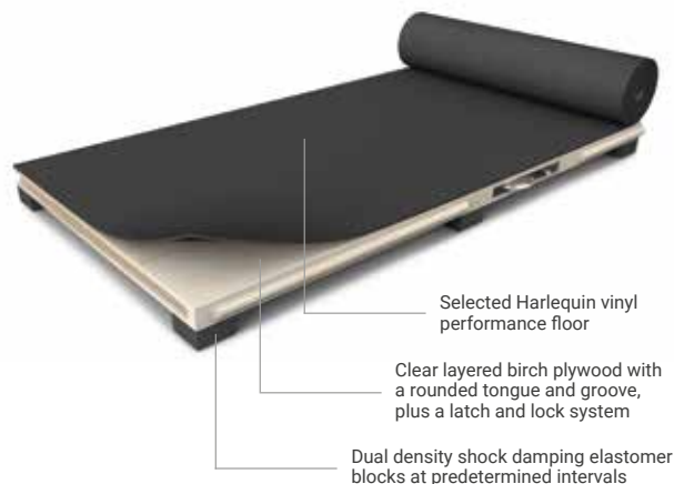
Harlequin latch and lock system
