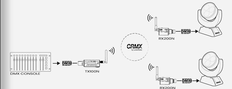
**CONNECT TX100N** features the new PoD (Power over DMX) technology that makes it possible to be directly powered through the XLR connector without the need for an external power supply. To take advantage of this feature, the TX100N must be connected to a PoD-compliant equipment.
