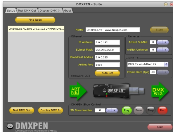
Figure 7: ArtNet -> DMX data direction selection
