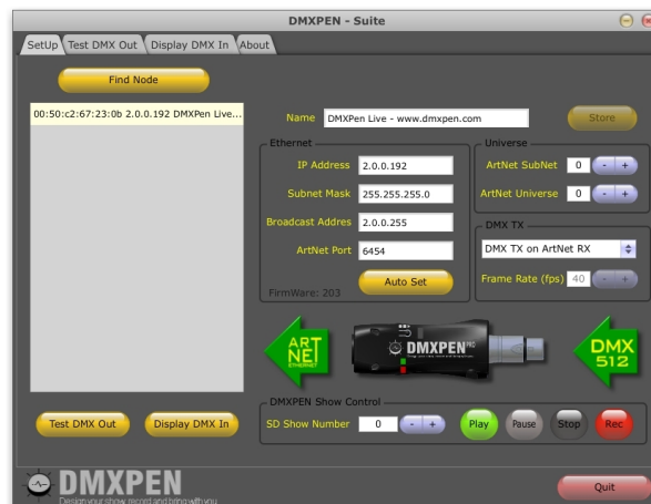
Figure 8: DMX -> ArtNet data direction selection
