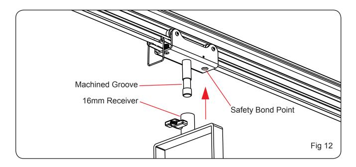
Carriages fitted with a 28mm Spigot are designed to accept equipment fitted with a 28mm Spigot. The receiver has 3 safety points incorporated in its design.
