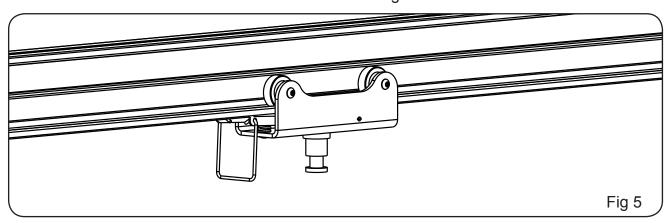
f. T84205 - 6 Wheel Carriage - 28mm Receiver - SWL 100 Kg
