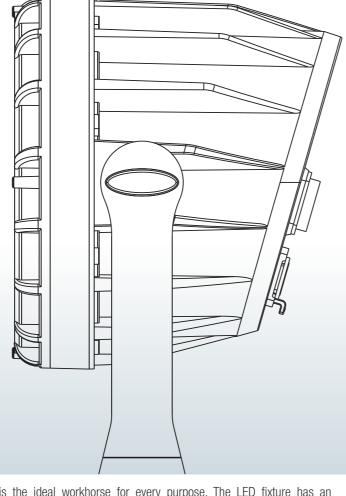
The CLF Yara is the ideal workhorse for every purpose. The LED fixture has an outstanding smooth RGBW color mixing delivered by a 14 high power LEDs with a very punchy 15° beam angle. The special selected LED provides high output with intense colors and an exceptional white balance. IP65 rating makes the Yara suitable for both in- and outdoor use.
