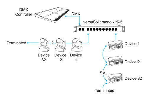
In this example, the maximum number of DMX devices are driven on outputs 1 and 10.
