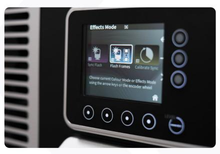
The Vortex8 is now calibrated. It can now be set to desired effect mode (Normal, Strobe etc) E.g. Select Effects > Flash Frames.
