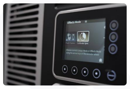
2 Select Effects > Calibrate Sync. The fixture will start to flash at the locked framerate (see **5.20 Calibrate Sync** for more details on these settings).
