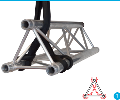
TRIANGULAR TRUSS | APEX UP 2 SLINGS, CHOKES ON BOTTOM CHORDS
