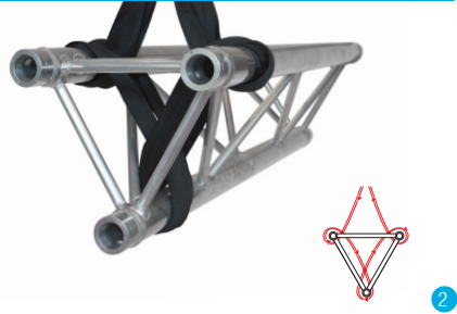
TRIANGULAR TRUSS | APEX DOWN 1 SLING, BASKET ON BOTTOM CHORD AND WRAPS ON TOP CHORDS
