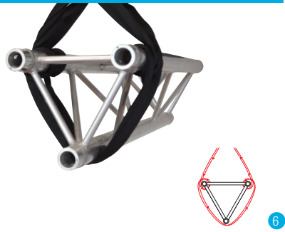
TRIANGULAR TRUSS | APEX DOWN 1 SLING, BASKET WITH WRAPS ON TOP CHORDS
